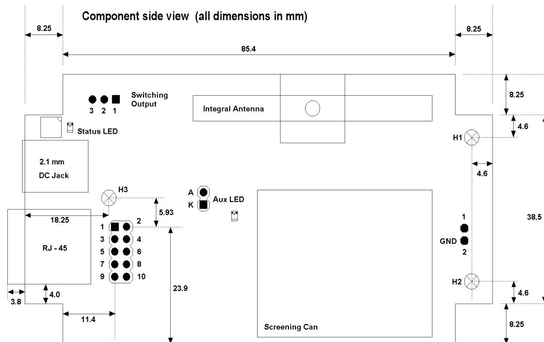
H1..H3: fixing holes (3.2 mm dia for M3 screws)
